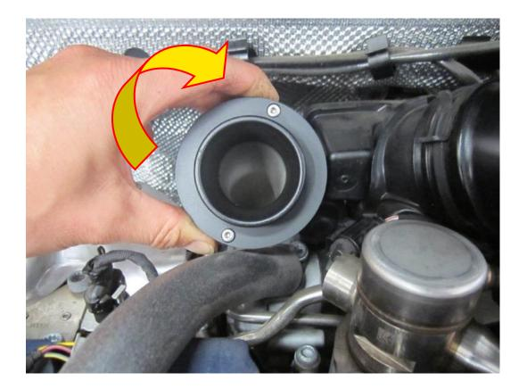
Fit the Forge Motorsport silicone hose into place and secure it with the two hose clamps supplied, 70-90mm clamp on the larger end of the hose and 40-60mm on the smaller end. Use a 7mm socket and rachet to tighten the clamps.
