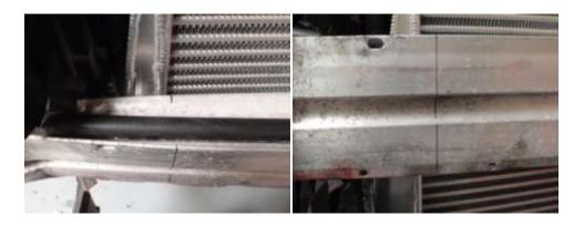
23. Mark 25mm outward of the line. On both sides of the crash bar.
