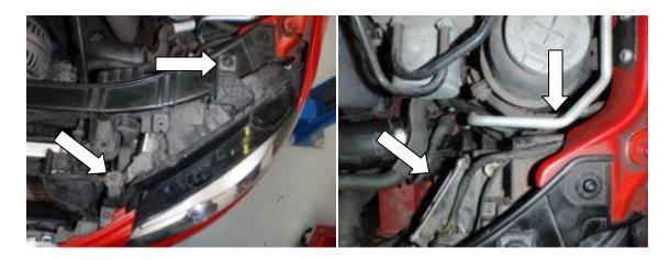
9. Once these have been removed the headlight can be pulled forward and twisted to clear the body to free it from the vehicle. Place the headlights in a safe place to prevent damage while working on the car.
